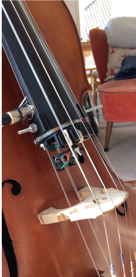
Fig. 4. An analogue Feedback Cello with each string gain being adjusted manually on an off-board mixer. See https://youtu.be/2UX6BwJMTHs
